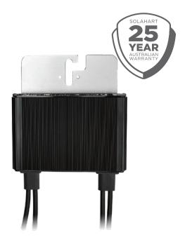
The SolarEdge Power Optimiser is a DC/DC converter that connects to a single panel to monitor and control its individual performance. This level of control mitigates panel mismatch losses due to partial shading and improves the performance of the PV system. It also allows for more flexible system designs and greater roof space utilisation.
